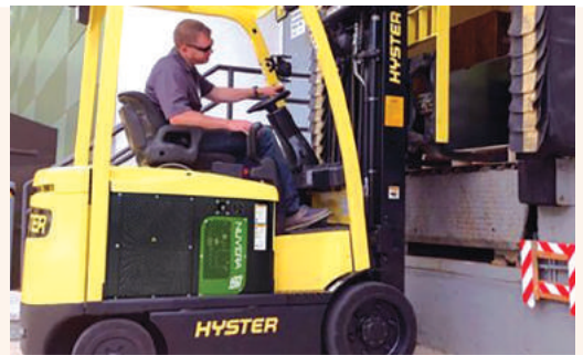
Hyster® fuel cell-powered forklift. Image credit: Hyster-Yale Group
