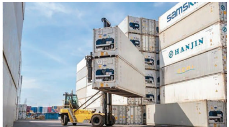
Hyster® top-loading container handler. Image credit: Hyster-Yale Group
